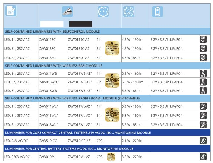
All versions also available as COOL-luminaires with external battery housing for mounting within the building. The luminaire may be mounted outside or in cool stores
