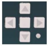
Even without an external input or control device, navigation through the menu structure of the system software is no problem thanks to the 4-way navigation buttons.
