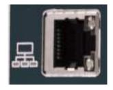
The Ethernet interface integrated in the control unit enables the system to be completely configured and monitored via a web interface.
