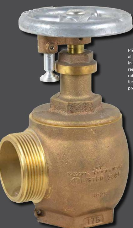
Pressure restricting valves from Elkhart Brass all feature rugged cast brass construction in your choice of finishes. The pressure restricting valves feature rubber seats and are rated for use at 175 psi (12 BAR). Although factory setting is recommended, all the pressure restricting valves are field settable.
