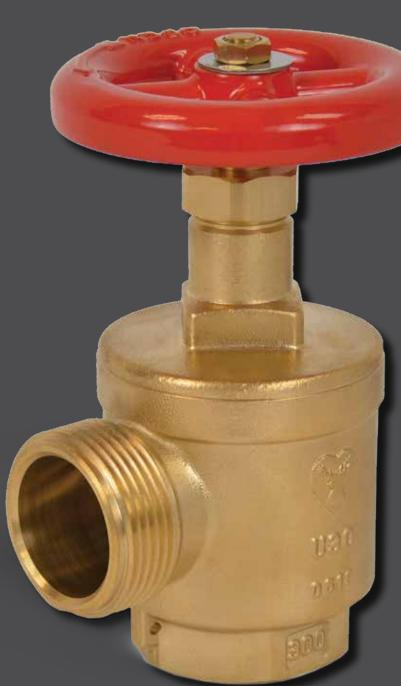
The Elkhart Brass U angle valves are used in firefighting piping systems as Fire Department outlet connection or Fire Hose Rack assembly connection. They are available in 1.5" and 2.5" inlet/outlet sizes and offered in angle style with NPT and NHT threading options. The U valves are UL Listed and FM Approved.
